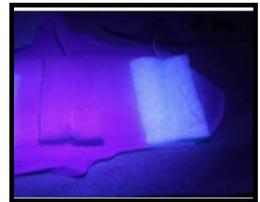
Note: If an intermittent discharge is suspected, the cotton pad can be secured at the outfall or an upstream point (such as suspended in a storm DI) for a given length of time during dry weather before black light exposure.
