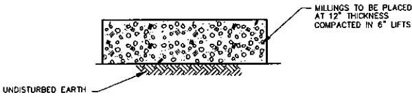
PARKING LOT PAVING DETAIL NOT TO SCALE
